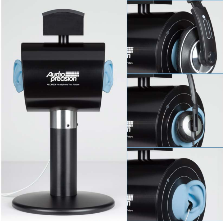
Figure 6. Audio Precision AECM206 headphone test fixture.
